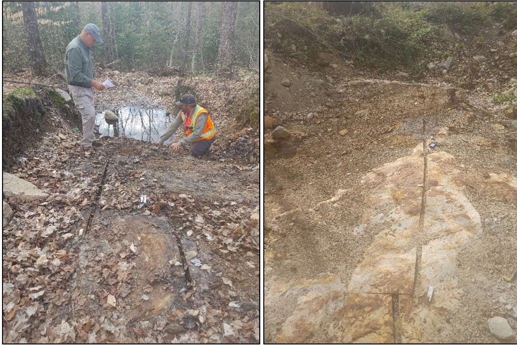
Figure 12-10: Representative trenching and channel sampling at Standard
