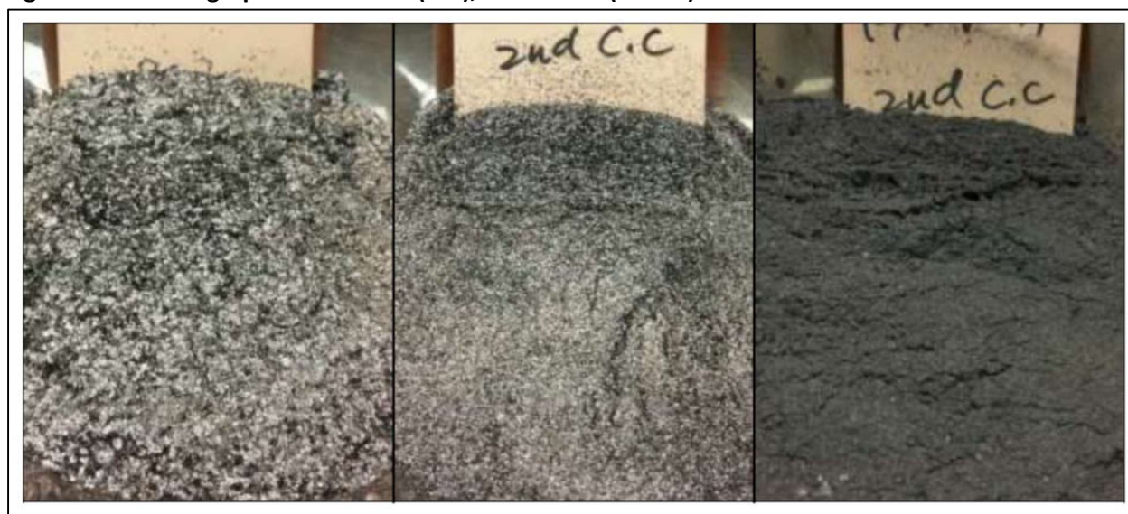
Figure 13-4: Photograph of +48 mesh (left), +100 mesh (centre) and -100 mesh concentrates
