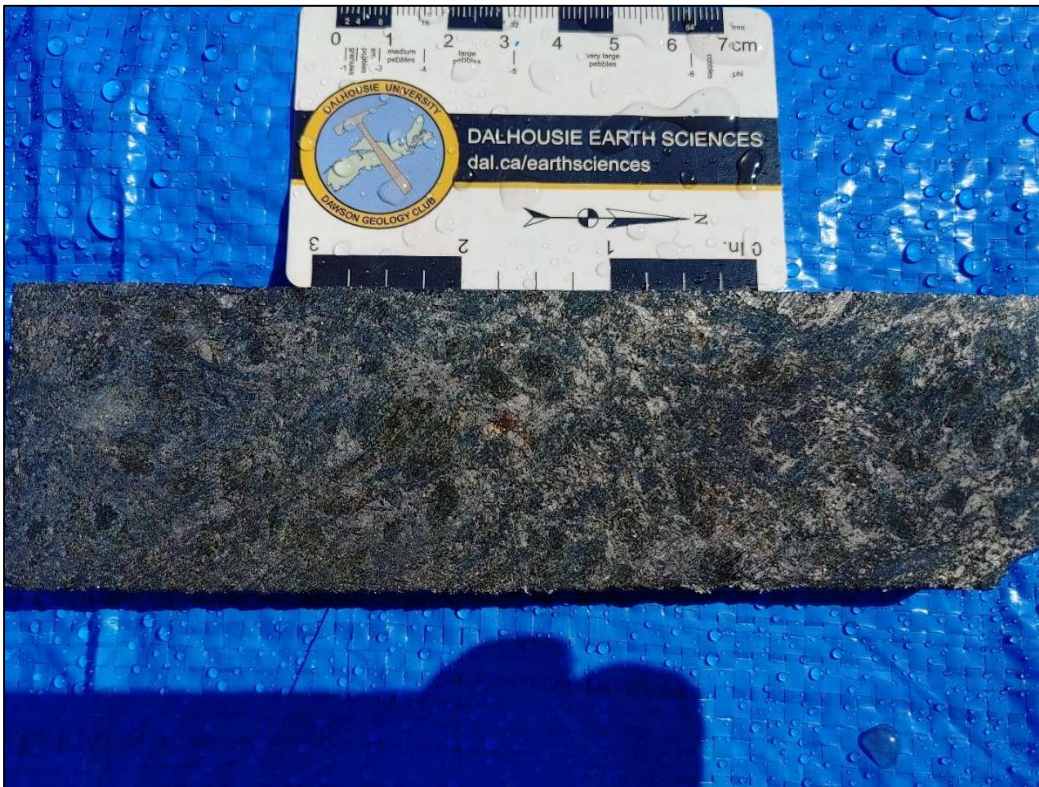
Figure 7-7: Graphite mineralization within the host recrystallized limestone – marble unit (LB-23-56, LAB Property)
