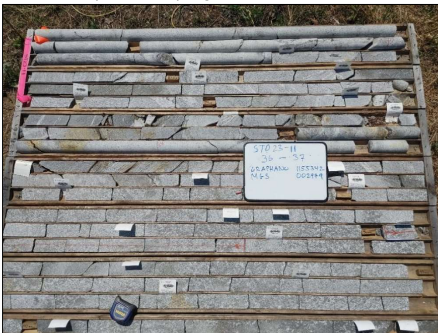
Figure 12-7: ST23-11 – 12 m recrystallized limestone unit with coarse disseminated graphite and minor units of quartzite and paragneiss
